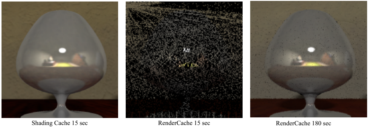
Figure 7: Equal time and equal quality comparison between our system and the RenderCache for glossy reflections
